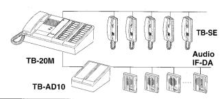
In place of TB-SE handset subs, TB-M master may have max. 10 door stations, by using a TB-AD10 adaptor.
